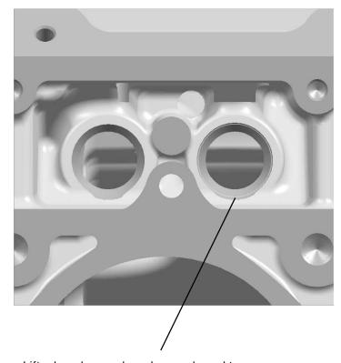
Cam bore material has been added to accommodate a 68mm (2.677") bore (shown) for 60mm roller cam bearings. Interrupted cutting will be experienced when machining to 68mm.
