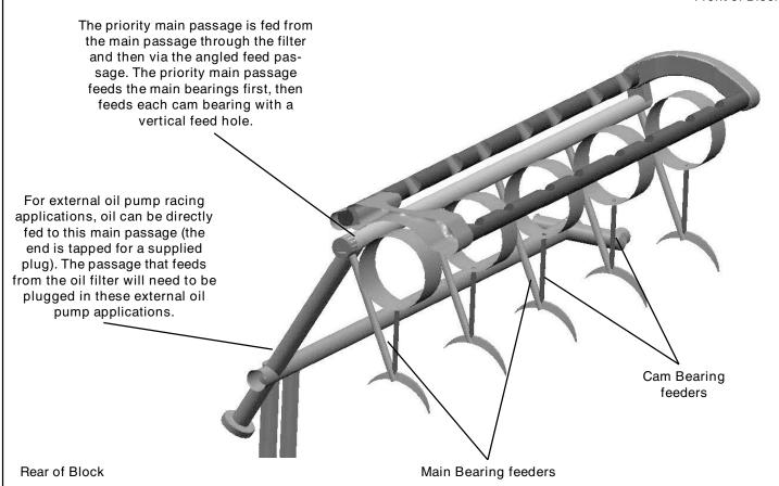
The priority main oiling system was specifically designed to accommodate 60mm cam journals, as well as mechanical and oversized lifters or lifter bushings (all of these require appropriate machining). This design ensures uninterrupted oil supply to the mains and guarantees oil supply to the main bearings first, not only upon startup, but also in the event of pump starvation. The oil must pass through the main passage before it fills the lifter galleys.
