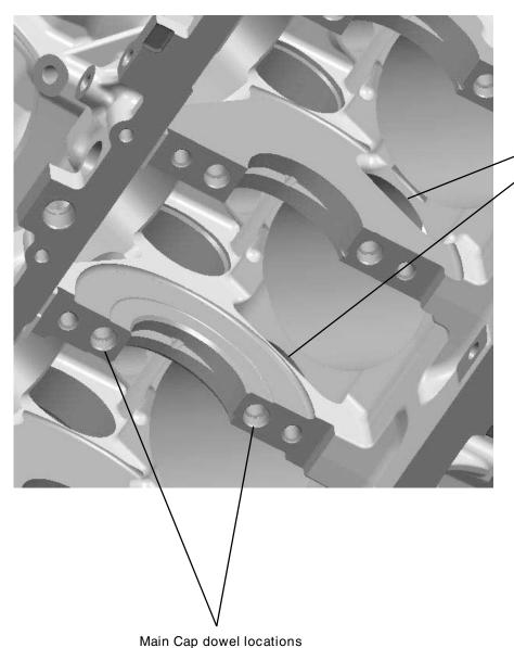
Bay-to-bay Breathing windows in the main caps show significant HP gains at higher RPMs without sacrificing block integrity
