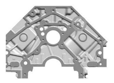
The 7<sup>th</sup> transmission mounting hole has been added to the block. It intersects one of the head bolts when machined at full depth, so the tap depth has been reduced to eliminate this. When it is to be used, a shorter stud (recommended) or bolt will be needed.
