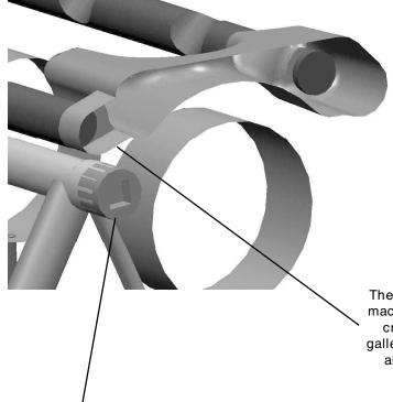
The left lifter oil feed passage is machined to intersect the cast in crossover between the lifter galleys at the rear of the block to allow for pressure and flow equalization.
