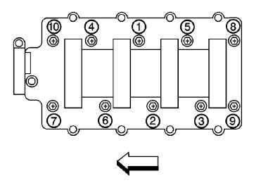
Crankshaft Bearing Cap Bolts and Studs (arrow indicates front of engine)
