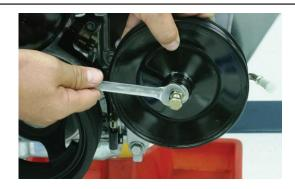
8. Using two wrenches hold the bolt and tighten the nut against the washer to press the pulley onto the shaft. The pulley is completely installed once the outside of the pulley hub is flush with the end of the pump shaft (see picture below)
