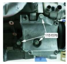
Install A/C Compressor 25891791 using (3) 11516109 (long) and (1) 11516503 (short) bolt and torque to 50 Nm (37 lb ft).
