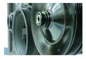
Install Generator using (2)11516360 bolts and torque to 55 Nm (41 lb ft).
