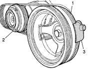
Install Power Steering Pump Brace 12554032 to rear of pump using (2) 11514597 nuts and torque to 50 Nm (37 lb ft).
