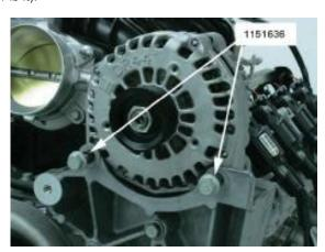
10. Install Idler Pulley 12580771 on bracket boss below Generator as shown. Torque bolt to 50 Nm (37 lb ft).
