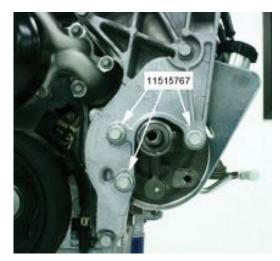
6. Install brace bolt 11515764 to block and torque to 50 Nm (37 lb ft).
