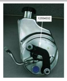
Install Power Steering Pump to bracket using (3) 11515767 bolts and torque to 50 Nm (37 lb ft).
