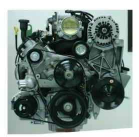
NOTE: If you are installing Air Conditioning, it is recommended to install the A/C compressor, bracket and belt before installing the main drive belt. If you are not using air conditioning, skip the first 3 steps and begin on step 4.
