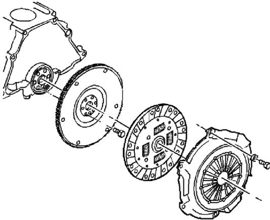
2. Remove the clutch cover bolts one turn at a time, until spring pressure is relieved.
