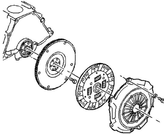
1. Install the clutch disc and the clutch cover.
