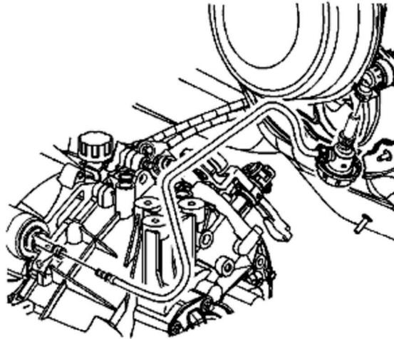
6. Connect the clutch actuator cylinder line.
