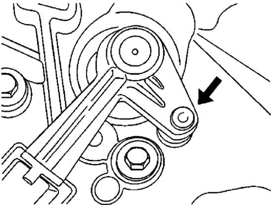
4. Install the upper line release bolt.
