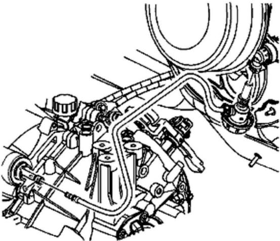
1. Disconnect the clutch actuator cylinder line.
