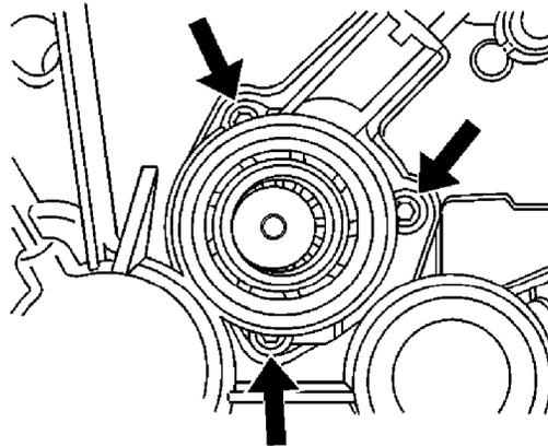
3. Remove the clutch actuator cylinder bolts from the transmission.
