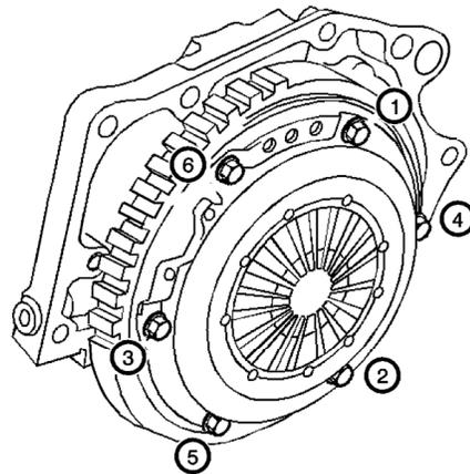
4. Tighten the clutch cover to flywheel bolts in the sequence shown. Tighten the bolts to 30 Y (22 lb ft).
