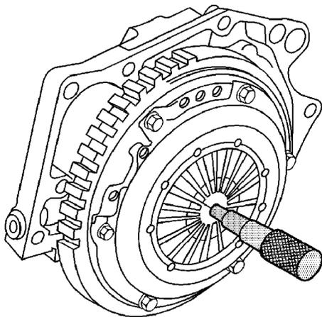
3. Install the Pilot tool in order to support the clutch cover to flywheel assembly.
