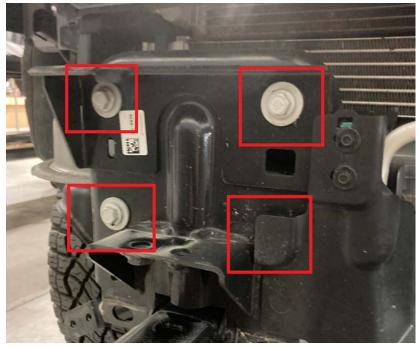
4. Install AEV-provided green push nuts into front of upper frame brackets, then install Air Baffle using M4.2x25 screws.
