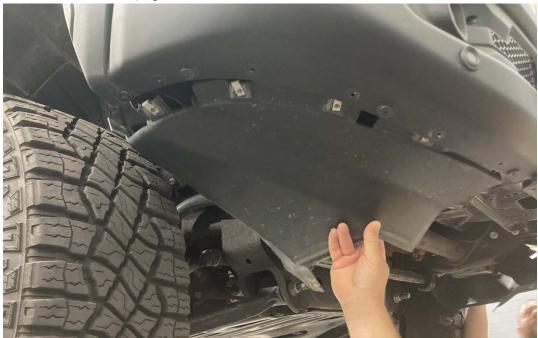
11. Install radiator skid plate available separately. Refer to skid plate instructions for process.
