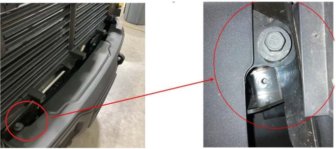
b. From below, install 4 lower M12x30 washer head bumper bolts from AEV hardware kit.
