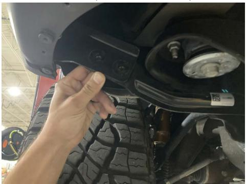
7. Install center bumper molding. (Note: Not used with winch kit)
