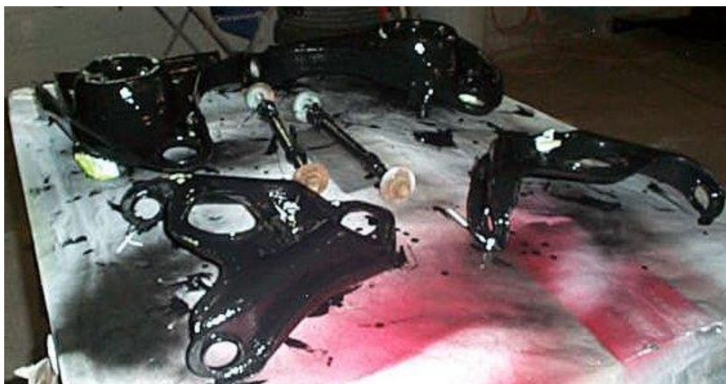
Control arms painted and ready for reassembly
