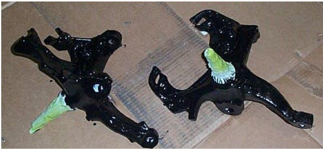
Spindles painted and ready to be installed
