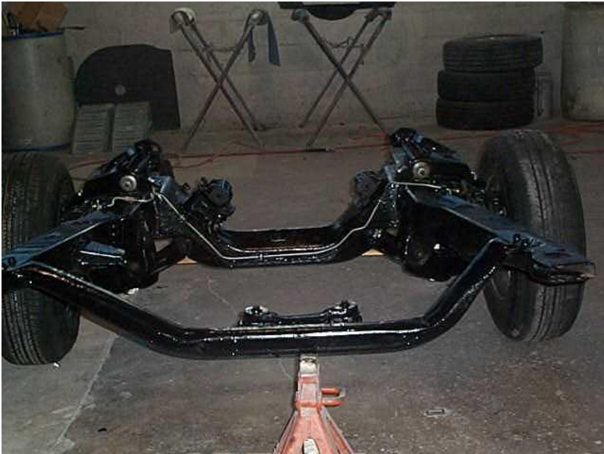
Complete with new brake lines the frame is all ready for install
