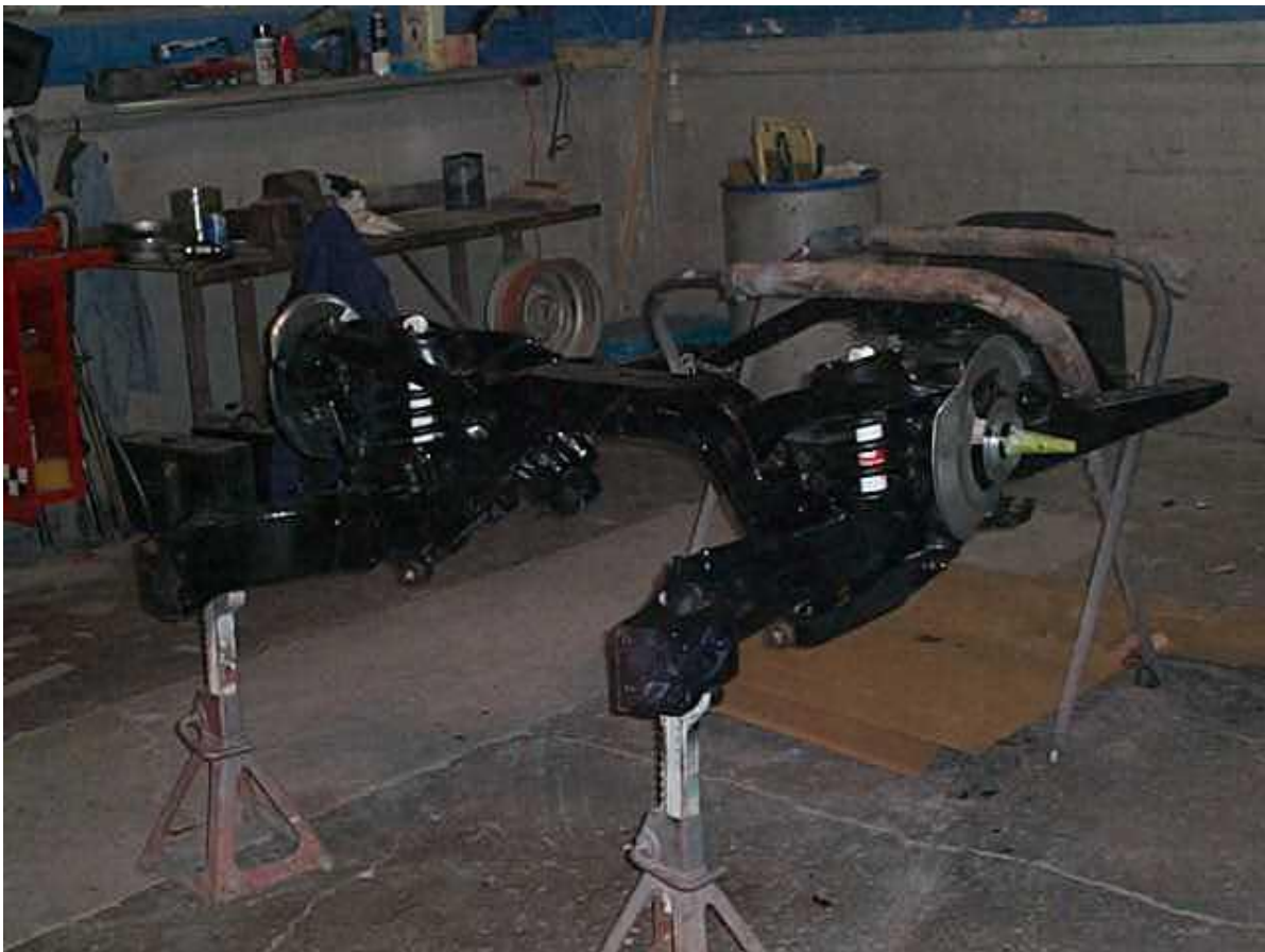
Springs, shocks, spindles installed 1
