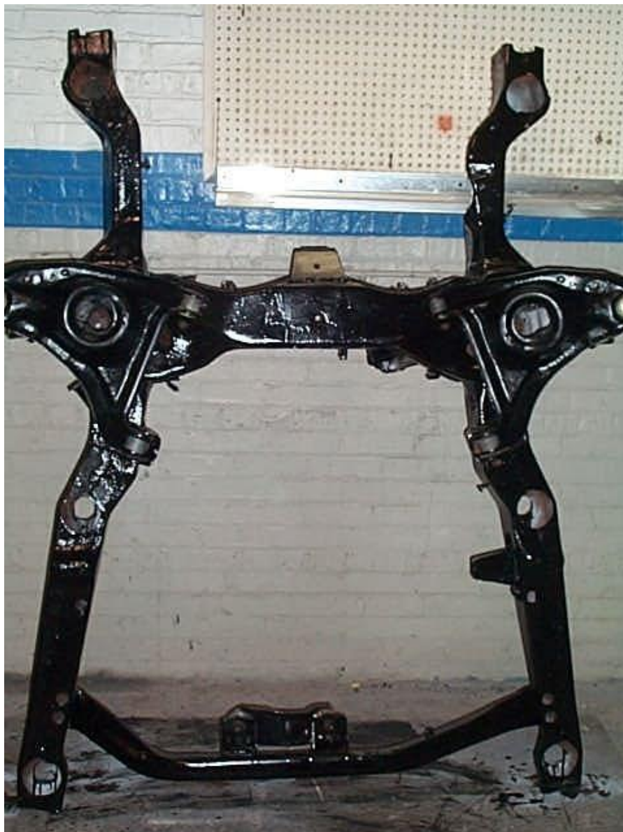
Sub-frame, sanded, cleaned, painted, control arms mounted 1
