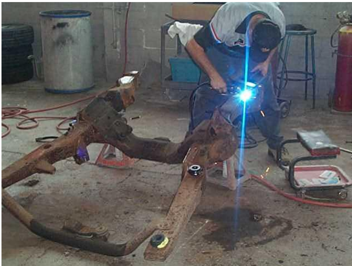
Repairing body mount holes with new steel
