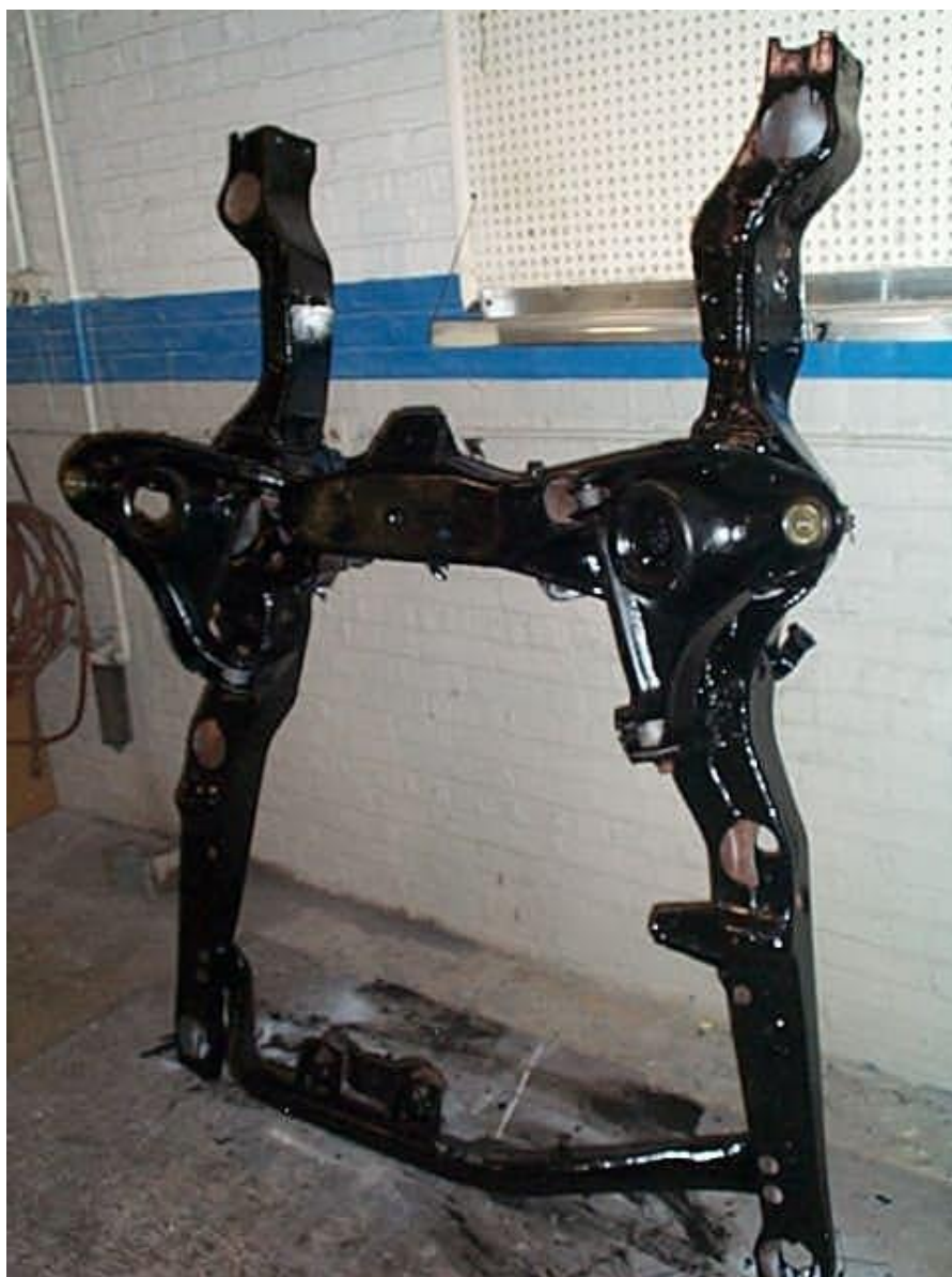
Sub-frame, sanded, cleaned, painted, control arms mounted 2
