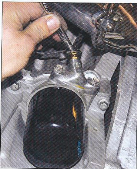
The bypass adapter and sending unit is installed. Each brand of sending unit typically has its own thread size. You need to use the size to tap the unit. (Street & Performance)
