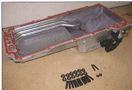
For the LS7, ATS offers this pan for the 1967–1969 F-body cars with the ATS engine mounts. If you flip the ATS engine mounts upside down, this pan can be used in 1964–1967 GM A-body cars as well. (ATS)
