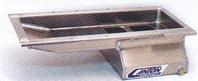
The Canton aluminum drag race oil pan for LS engine swaps fits GM A-, F-, Y-, and 1970s X-body cars. It is an aluminum sheetmetal pan, with trap door baffles for oil control. The required remote filter adapter is included. (Canton Racing Products)
