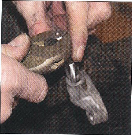
The plug is tapped to match the threads. Cutting oil makes the tapping process easier and keeps the aluminum from galling on the tap. (Street & Performance)
