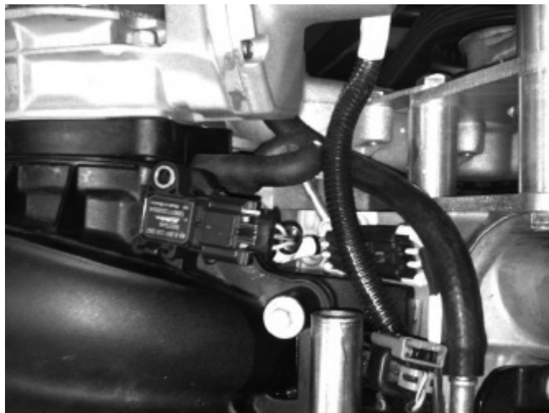
Figure 2 Re-install O'ring and install MAP sensor. Lubricate lightly with engine oil. Plug in MAP sensor using jumper provided with Engine control System kit. See Figure 3.
