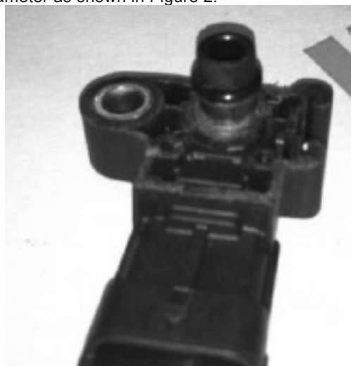
Figure 2 Re-install O'ring and install MAP sensor. Lubricate lightly with engine oil. Plug in MAP sensor using jumper provided with Engine control System kit. See Figure 3.
