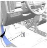
17. Pull back driver front side door sill garnish molding (1) and remove side kick panel to route wire.
