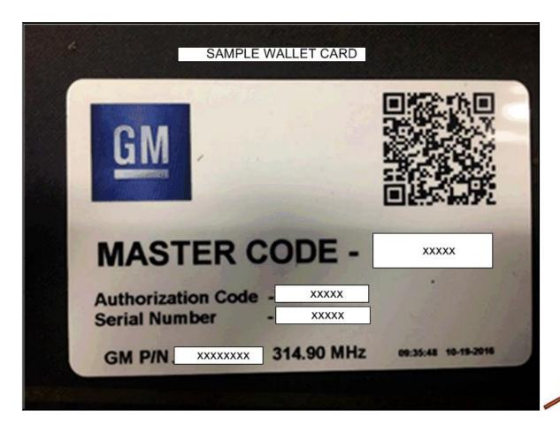
1. Technician use a QR/Bar (QRB) Code reader and scan the QRB code from the Keyless Entry Keypad Wallet Card. You can also take a picture of the QRB code.
