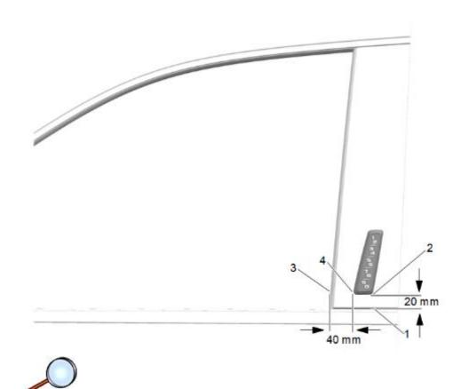
1. **Driver Side Front Door:** Starting from the top driver side front door window belt reveal molding (1) measure 20 mm up and position keypad (2).
