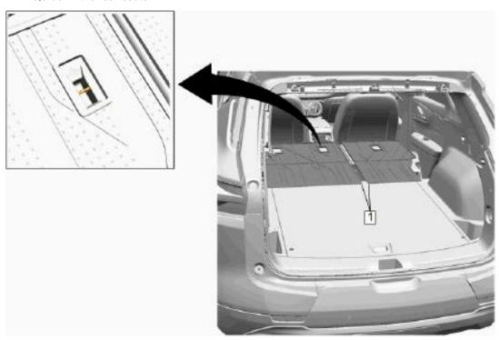
2. Install the seat back cargo tray pieces (1). Align the tether openings to the seat tether anchors, as shown. Apply pressure to secure the Velcro patches to the seat backs.
