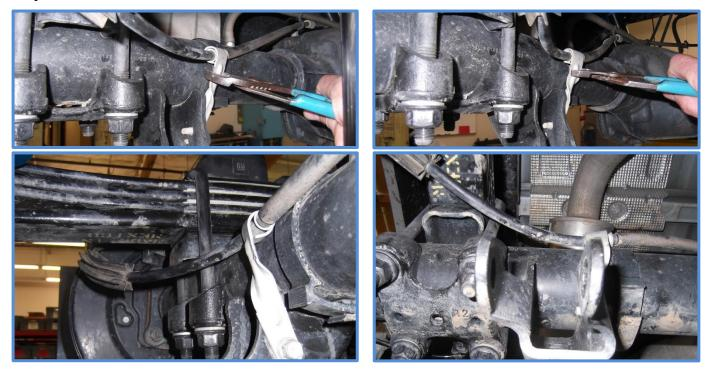
3. Install King Shocks reusing the factory hardware. Shocks are side specific and need to be oriented with the long offset spacer towards the outside of the vehicle and reservoirs towards the rear of the vehicle. See Photos...
