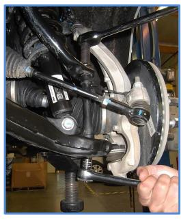
5. Remove the nut from the Upper Control Arm ball joint using an 18mm socket and separate the UCA from the upright.
