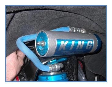
14. Install the provided hose clamps and secure reservoir to the reservoir bracket.
