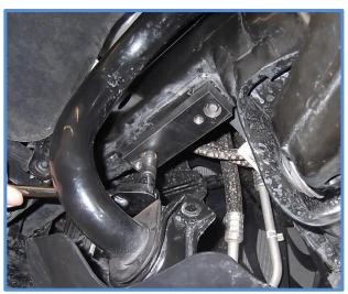
17. Bolt the sway bar to the sway bar plate using the supplied 3/8" x 3/4" bolts with a 9/16 socket.
