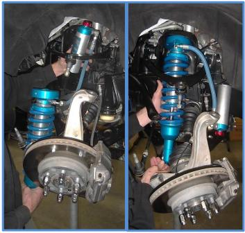
9. Install the factory bolt in the lower mount.
