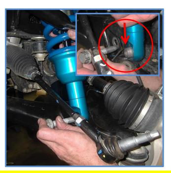
10. Jack up the lower control arm so that the upper mount on shock is tight against the upper mount on the truck (coil bucket). But not so tight that you can't move the shock around to line up the upper mounting holes.
