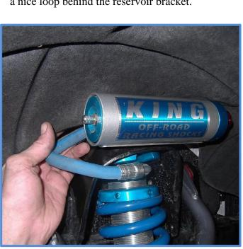
12. Twist the reservoir up so the hose is out of the way, line up the mounting holes and install the supplied 3/8" x 1" bolts. Start all the bolts by hand then jack up the lower control arm until the shock is tight against the upper mount. Use a 9/16" ratchet wrench to tighten the upper bolts.
