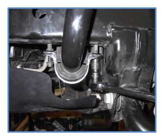
16. Using the factory bolts, attach the sway bar plates to the frame with the threaded holes towards the front of the truck as shown below.
