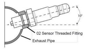
Mark the drilling location on the exhaust system pipe with a permanent or paint marker. Check the proposed mounting location to ensure the clearance for the O2 sensor is adequate and that the O2 sensor connector on the main harness will reach the O2 sensor location. Make sure to take engine movement into consideration when checking for clearance.
