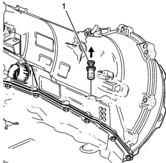
**Note:** It may be necessary to use a long pair of 90 degree needle nose pliers to lift the plunger and remove the plug assembly.
