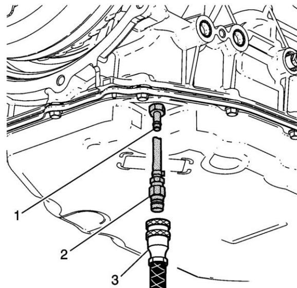
Install the DT-51190 fluid fill pan adapter (1) and, if necessary, one adapter from the DT 45096-30 cooler flush adapters (2).
