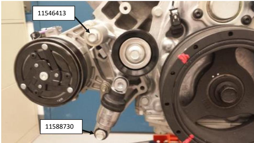
4. Install generator 84331091 using (2) 11546413 bolts. Torque to 54 NM (43 lb ft).
