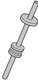
Install the oil priming tool, Melling part number PT13 or equivalent. The lower collar on this type of priming tool directs oil flow to both banks of cylinders. Do not attempt to prime using only a shaft to turn the oil pump.
