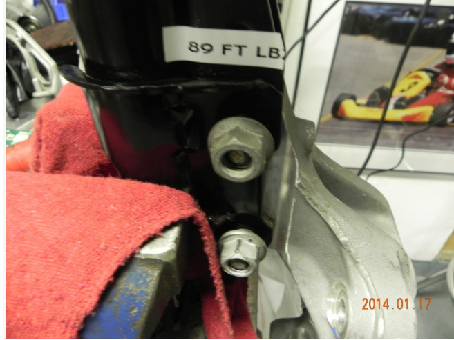
EVEN THIS FAR OUT CAN LEAD TO SPRING AND BEARING ISSUES. IT MUST BE POSITIONED CORRECTLY
