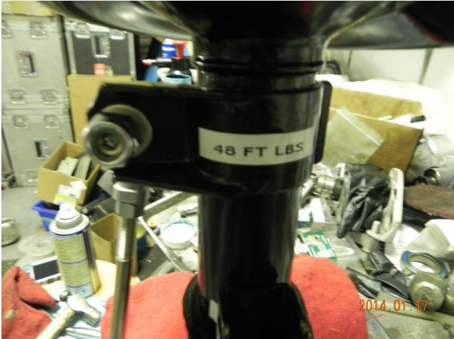
EVEN THIS FAR OUT CAN LEAD TO SPRING AND BEARING ISSUES. IT MUST BE POSITIONED CORRECTLY
