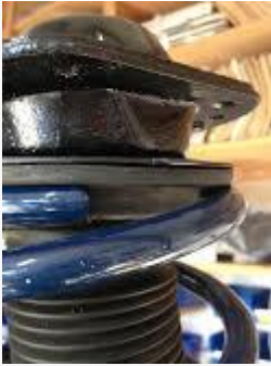
EVEN THIS FAR OUT CAN LEAD TO SPRING AND BEARING ISSUES. IT MUST BE POSITIONED CORRECTLY
