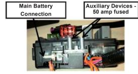
Attach a 12 volt ignition switch feed from the vehicle to the pink ignition switch wire in the harness (this is required to enable the proper powerup sequence of the ECM). This can be routed into the passenger compartment with the accelerator pedal connector and diagnostic link connector. Next, connect battery power (minimum 8 gauge wire) to the horizontal stud on the fuse relay center The other two studs are for accessories and are 50 amp fused), and the harness installation is complete.
