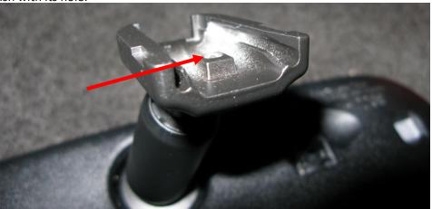
Slide the base of the mirror down onto the mounting hardware which was left on the windshield.
