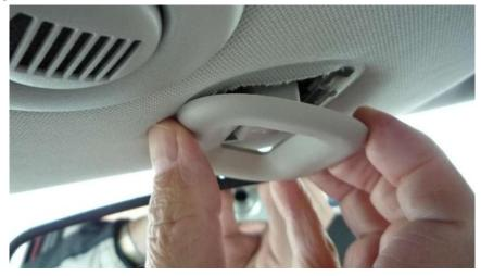
Finally, pull the driver side of the trim down. Here is a picture of the tabs on the trim to give you a better idea of what is keeping it in place:
