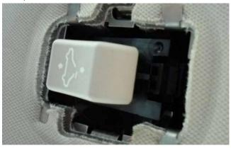
Finally remove the switch by simply pulling it the rest of the way out. There will be a wiring harness snapped into the passenger side of the button and it may be taped to the headliner. This may make it slightly difficult to pull down enough wire to work with.
