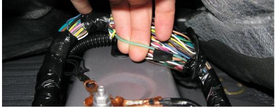
\*\*IMPORTANT\*\*: I suggest you check to be 100% sure that you have the correct wire before you tap into it. You can check by inserting a needle through the insulation and into the wire. Then put your car into reverse and measure the voltage between the needle and a ground point. This will help to prevent taping into the wrong wire and causing problems.
