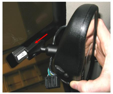
Tighten the Torx screw to secure the mirror to the windshield.
