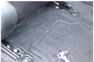
With the bolts removed, pivot the driver seat forward and disconnect the plug on the bottom of the seat cushion.
