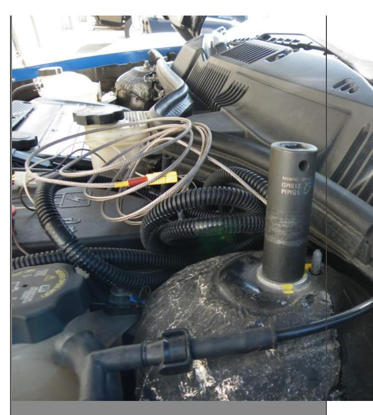
remove strut to knuckle cross bolts ( takes a hammer to knock them out as they are a spline fit in the knuckle dont damage the threads, put the nut back on if you are a clumsy ijiit or use a center punch) undo abs connector remove abs wire retainer plate and remove strut. Be carefull not to pull back on rotor as you will pop the axle out of the trans and spill fluid like I did. (Put a drain pan out next time, Qwik)
