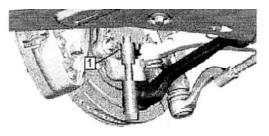
15. Use the CH-42188–B separator (1) to separate the front lower control front link from the steering knuckle.
