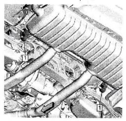
7. Install the two rear exhaust muffler isolators.
