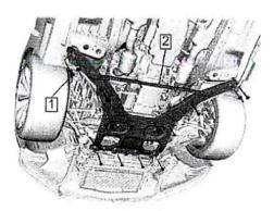
20. Front Cradle Shear Plate Fastener (1) » Remove
