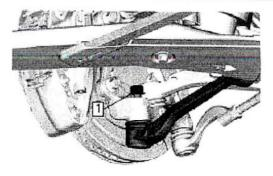
14. Steering Knuckle Nut (1) » Loosen
