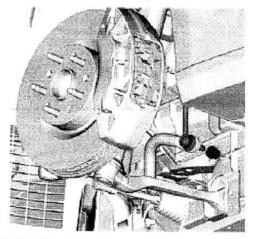
22. Front Stabilizer Shaft Link Nut (1) @ Stabilizer Shaft » Remove
