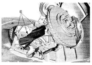
2. Front Brake Rotor Cooling Duct Deflector Bolt (1) » Remove [3x]
