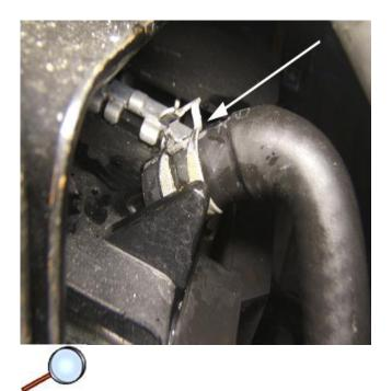
**Important:** The tapered end of the check valve must face the nipple on the radiator. A check valve in the horizontal position will not function properly.
